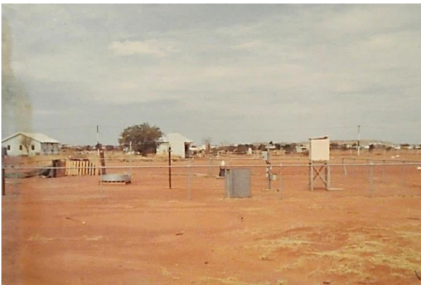
Figure 4. The Cloncurry Aeradio weather station in October 1965 comprised of a standard 230-litre Stevenson screen (right), an A-pan evaporimeter suspended off the ground on a pallet but apparently without a bird-guard, a copper-clad Dines pluviometer in the background (used to record rainfall intensity), and a standard 8-inch (203 mm) raingauge. Note that the site is dusty and bereft of groundcover. (Photograph courtesy of CAHS.)
